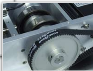
The Prep-250 features a servo motor, belt drive and reliable eccentric cams.
